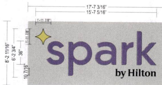
CHANNEL LETTER W/ BACKER PANEL DETAIL SCALE: 3/16" = 1'-0"
