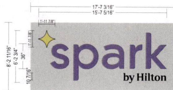
CHANNEL LETTER W/ BACKER PANEL DETAIL SCALE: 3/16" = 1'-0"
