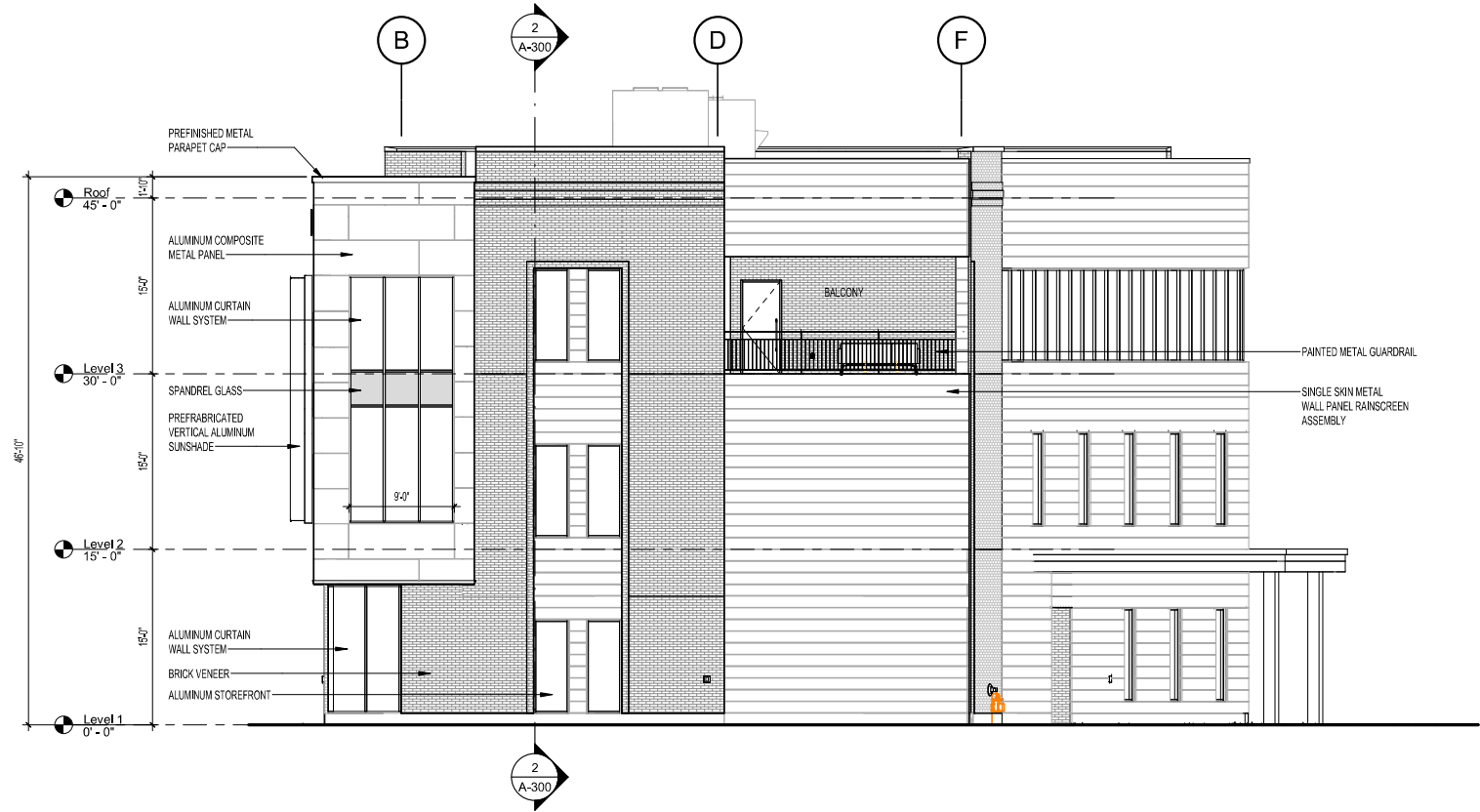
1 BUILDING ELEVATION - NORTH 1/8" = 1'-0"
